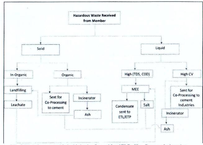
M/s. BEIL Infrastructure Limited is having Secured Landfill Facility, Common Incineration System and Multiple Effect Evaporator (MEE) Plant. In the developed portion of secured landfill, BEIL INFRASTRUCTURE LIMITED is receiving waste according to the acceptance criteria for secured landfilling. If waste does not meet criteria for direct landfilling, necessary treatment like neutralization / stabilization etc. is given. The developed portion of secured
